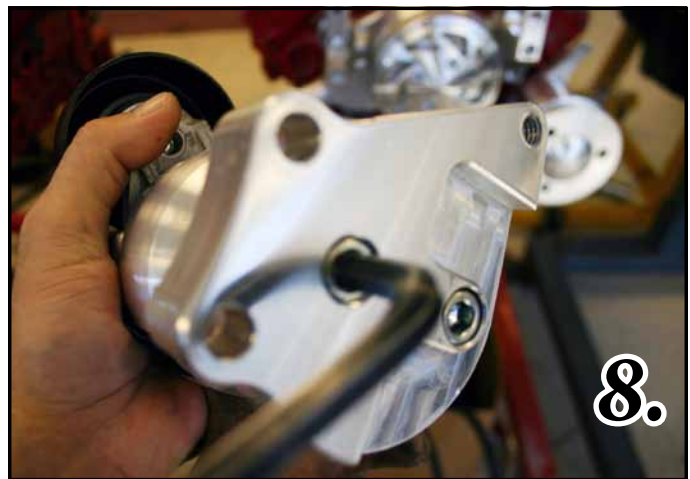
Photo-8 1. Hold Tensioner Body in a vise to remove bolt & washer from tensioner pulley. Note: Bolt is a left handed thread, turn clockwise to remove. Install the Tensioner into the 20256-B Bracket cover use a \frac{3}{8} x 3\frac{1}{4} " SHCS and install the (781-A) cover as shown and bolt into place.
