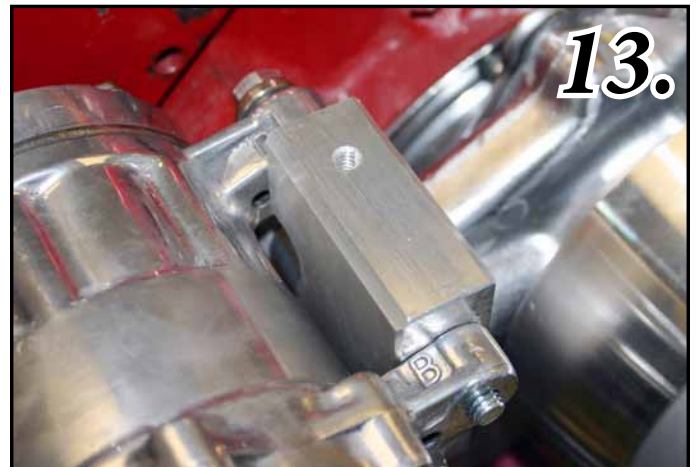
Photo13 Mounting the A/C Unit. Remove the A/C bracket ear from the water pump leaving a Alt ear on tight, thru the rear ear of the A/C unit use a M8 x 120mm hex bolt then reinstall the A/C ear to the water pump.
