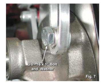
8. Mount power steering pulley to power steering pump shaft. Check power steering pulley to crank pulley alignment. Install belt (*Use 39.5" 5 rib serpentine belt for serpentine conversions*) and adjust belt tension by pulling up on the power steering pump. Belt tension is correct when there is no more than ¼" play in the belt at midpoint between the power steering pulley & the crank pulley. Lock the belt tension by tightening the adjustment bolt with a 9/16" opened end wrench (fig. 8).
