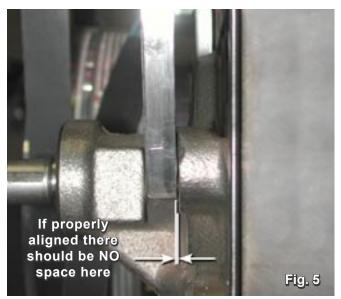
**Important Note:** Due to variations of water pump boss castings particularly in aftermarket and polished pumps it may be necessary to add spacer washers between (20176-*A*) Front Support Bracket and the water pump boss. (fig. 6) if this should be required it will also be Onecessary to place a second spacer washer between the (20176-B) Rear Support Bracket and power steering pump. (fig. 4)
