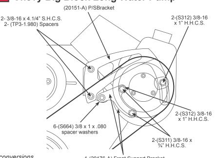
1-(20176-A) Front Support Bracket 1-(20176-B) Rear Support Bracket
