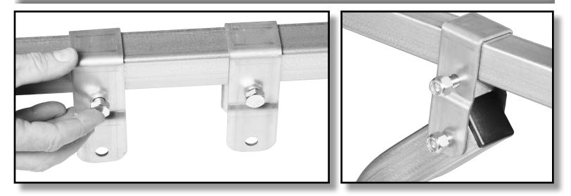
16. Install the D-Rings to the ends of the load bars. Slide a nylon lock nut into the open end of the load bar and align with the hole. Place washer under bolt head and insert it through the D-ring.
