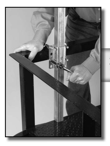
9. Assemble the bottom plates as shown using the square U-bolts and nuts, no washers here.
