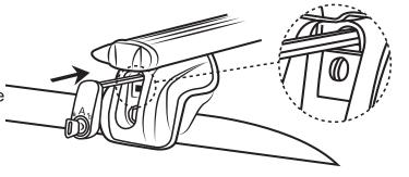
6). A U-bolt or a T-bolt (not included) are typically used when fixing other roof top items onto your roof bars. If using a T-bolt simply open the end cap, slide the T-bolt into the cavity then close the end cap.
