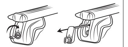
2). Remove the allen key from its storage position (the top opening). Insert the allen key into the bottom opening and twist anti-clockwise to open up the clamping area..
