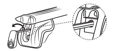
3). Position the roof bars 700mm apart on the roof rails (unless different instructions are given by the vehicle manufacturer).
