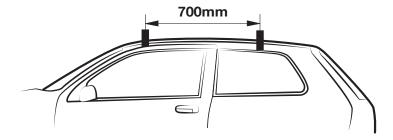
Warnings / Limitations: The load you are carrying plus the weight of the rack must not exceed the maximum weight limitation of the vehicle's factory raised side rails. Before installing, confirm your vehicle's factory specifications.
