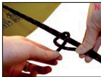
Form a knot with the free end and tighten. Form a second knot for safety purposes.
