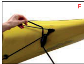
Keeping the rope tight and S-hook in place, thread the free end up and through a strong point on the kayak
