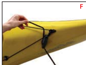
Keeping the rope tight and S-hook in place, thread the free end up and through a strong point on the kayak
