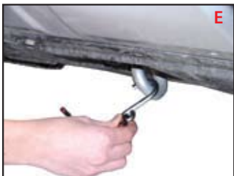
Attach S-hook to vehicle tow ring or other sturdy body part.
