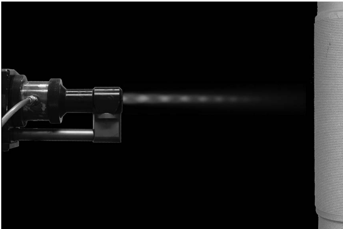
The MAHLE high velocity oxygen fueled thermal spray gun applying the patented HV385 ring face MAHLE coating.
