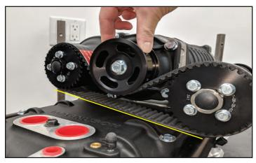
6. Press up on the lower belt span to ensure that it does not make contact with the upper belt. The upper and lower belt teeth should be about 4mm apart.
