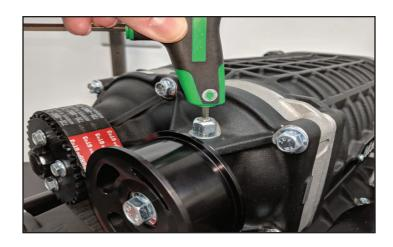
3. Remove the idler bolt shown with the arrow and apply Loctite 242 to the threads.
