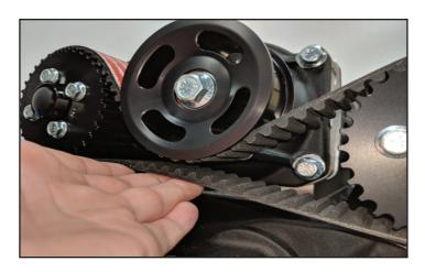
7. If the lower belt overlaps the upper one, as shown here, further adjustments will be needed.
