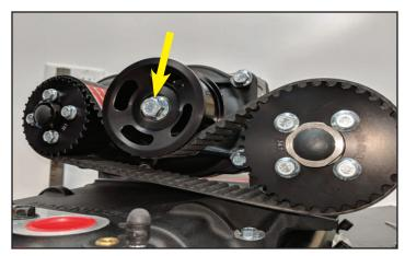
4. When reinstalling the "Idler Slide Nut" ensure that the rounded end faces up as shown in this photo. Reinstall the idler pulley with the idler bolt at this time.
