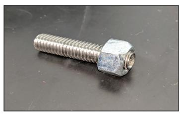
10. Tighten the set screw so it bottoms out against the Idler Slide Nut. If you need to adjust the belt tension you can loosen the idler nut and rotate the set screw 1/4 turn more or less to get the belt tension correct.
