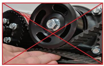
8. In this image the belt is too tight. Space between the upper and lower cog teeth is greater than 4mm.
