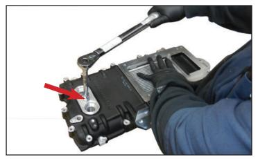
7. Intercooler to Upper Manifold: 18ft-lbs (Inspect Conical Washer – Found in Service kit 31-26-59-061)
