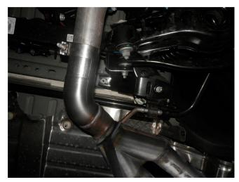
**Step 5.** Install the P/S Tail Pipe Assembly in the same manner. Leave all clamps loose for final adjustment of the system.
