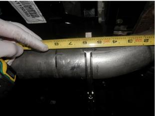
**Step 1.** It is necessary to cut the factory <u>exhaust system</u> to install the new Magnaflow unit. To do this measure 5.75" in front of the welds on the rear muffler inlets. Deburr the cut pipes to facilitate installation of the new system.
