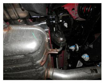
**Step 3.** Working front to rear disengage all welded hangers from the rubber insulators and remove the muffler assembly. (Retain the insulators as they will be needed to mount the new MAGNAFLOW system.) Once the OEM system is on the ground transfer both valve motors over to the new Magnaflow exhaust system using the OEM fasteners.
