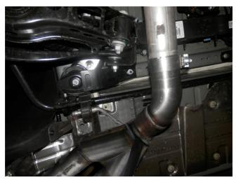
**Step 4.** Begin installation of the new system by sliding the D/S Tail Pipe Assembly inlet onto the cut outlet of the OEM exhaust and loosely fasten with the supplied 2.75" clamp. Fit the hangers into the rubber insulators.
