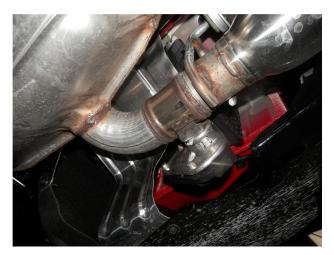
**Step 2.** Next you will need to unplug the electrical connection on the rear Exhaust Valve Control Motors (Qty 2) located on the OEM exhaust assembly.
