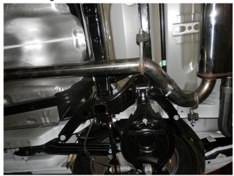
**Step 3.** Next loosely install the Extension Pipe Assembly and the Muffler Assembly using the supplied clamps. Engage all welded hangers to the rubber insulators.
