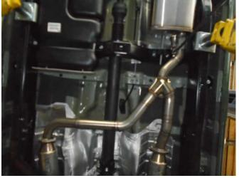
**Step 3.** Begin installing your new system by loosely attaching the Inlet Pipe Assembly to the drivers side catalytic converter outlet using the OEM hardware. Loosely slip the inlet of the Y-Pipe Assembly over the Inlet Pipe outlet and loosely secure with the supplied clamp. Loosely secure the Y-Pipe flange to the passengers side catalytiic converter using the OEM hardware.
