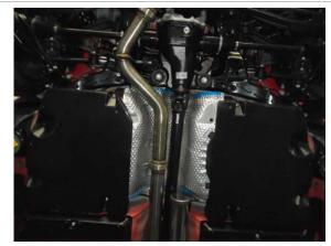
**Step 3**. Next, using the supplied 2.50" V-Clamp loosely attach the Y-Pipe Assembly to the Resonator Assembly and attach the hanger to the rubber insulator.
