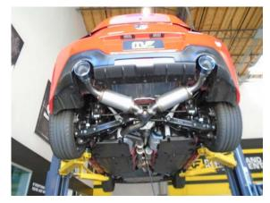
**Step 5.** Once a final position has been chosen for the new exhaust system, evenly tighten all clamps from front to rear using the torque specification on page one of these instructions. Inspect all flasteners after 25-50 miles of operation. Re-tighten if necessary.
