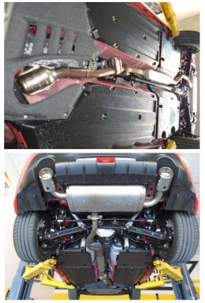
**Step 1**. Begin removal of your OEM exhaust system by unbolting the flange behind the catalytic converter. Remove all welded hangers from the rubber insulators. The exhaust can now be removed. Retain all fasteners and insulators asthey will be needed to mount your new MagnaFlow exhaust system
