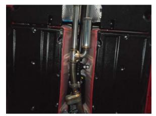
**Step 2.** Install your new system by first mounting the Resonator Assembly to the catalytic converter outlet using the OEM fasteners
