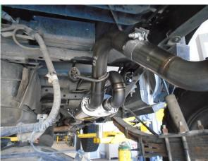
**Step 6:** Attach the Over Axle Pipe to the Muffler Assembly as shown using the provided 2.50" clamp and the OE rubber insulator.
