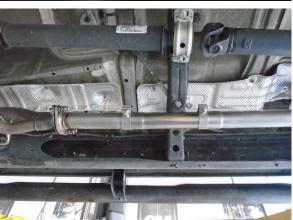
**Step 3:** Begin Installing the new system by attaching Inlet Pipe "A" to the vehicle using the OE Fasteners. - **NOTICE-** At this point On Crew Cab Long Bed vehicles you will need to add the provided 14" Extension Pipe using the 2.50" clamp.
