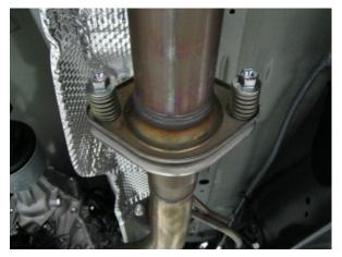
**Step 1:** To remove the OE exhaust system, unfasten the hardware at the inlet flange (Retain fasteners to be re-used).
