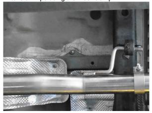
**Step 4:** Next, attach Inlet Pipe "B" to Inlet Pipe "A" (or the Extension Pipe) using a provided 2.50" Clamp and fit the hanger into the rubber insulator.
