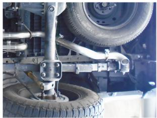
**Step 7:** Before installing the Tailpipe Assembly loosely fit the appropriate Hanger Clamp Assembly from the rear of the tailpipe. Hanger Assemblies are divided by year spread, 2005-2011 and 2012 -2015. Once fitted, install the Tail Pipe Assembly to the Over Axle Assembly using the supplied 2.50" clamp and fit the Hanger Assembly into the rubber insulator.
