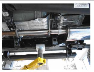
**Step 3:** Begin Installing the new system by attaching the inlet pipe to the vehicle using the OE Fasteners. and engaing the hanger into the rubber insulator.
