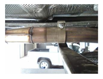
**Step 2.** Begin installation of the MagnaFlow system by attaching the X-Pipe Assembly with the supplied 2.75" clamps and fitting the hanger into the rubber insulator (Leave all clamps loose for final adjustment of the complete system.)
