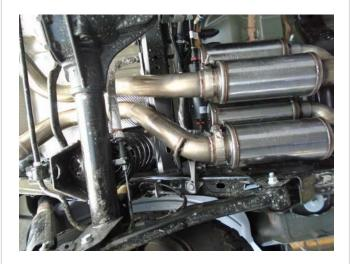
**Step 4.** Complete the installation by attaching the Tailpipe Assemblies onto the Muffler Assemblies using the supplied 3.00" clamps. Fit the hangers into the rubber insulators
