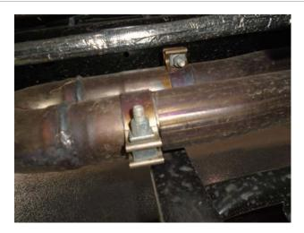
**Step 1.** Remove the OE system by loosening the clamps at the exhaust inlet. Extract the welded hangers from the rubber insulators and remove the exhaust. Do not damage the rubber insulators as they will be used to install the new MagnaFlow system.
