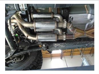
**Step 3.** Next install the Muffler Assemblies using the supplied V-Band clamps. Fit the hanger on the driver side assembly into the rubber insualtor.
