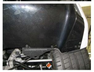
**Step 1.** To remove the OEM exhaust system you will first need to remove the rear valance. To do so you will need to remove The two 10mm bolts behind each reflector, the two 10mm bolts behind the license plate and two more 10mm bolts just underneath the license plate. Then you will need to remove the five 8mm bolts on both sides of the valance underside and remove it.
