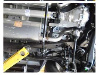
**Step 1.** To remove the OE exhaust system you will to need to remove the spare tire, heat shield and sway bar. Unfasten the clamp attaching the OE inlet pipe assembly to the catalytic converter. Do not damage or discard the inlet pipe clamp or rubber insulators as they will be re-used to mount the new system. Working front to rear disengage the hangers from their rubber insulators and remove the exhaust from the vehicle.
