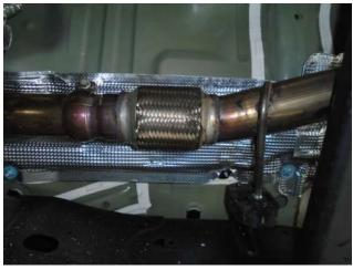
**Step 2.** To begin, fasten the Inlet Pipe Assembly to the outlet of the OE system using the OE clamp and by fitting the welded hanger into the rubber insulator (Leave all clamps and fasteners loose for final adjustment of the complete system.)
