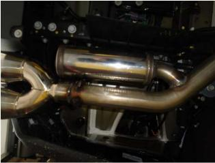
**Step 5.** Complete the installation by attaching both Tailpipe Assemblies to the Y-Pipe Assembly using the Supplied 2.50" clamps and fitting the hangers.
