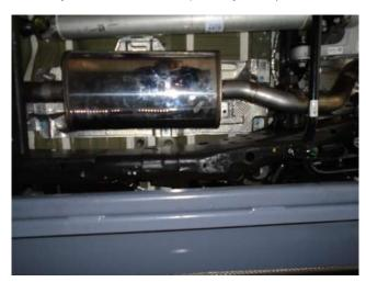
**Step 3.** Attach the Inlet Muffler Assembly to the Inlet Pipe Assembly with a supplied 3.00" clamp, fit the hanger into the rubber insualtor.
