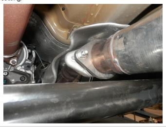
**Step 3.** Begin installation by loosely attaching the Inlet Pipe Assembly to the OEM flange outlet using the supplied hardware.
