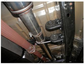
**Step 4.** Loosely install the supplied Hanger Clamp Assembly to either the Inlet Pipe Assembly or the Extension Pipe depending on your vehicles configuration. Locate the welded hanger to the forward rubber insulator as shown.
