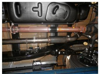
**Step 5.** Next loosely install the Muffler Assembly to the Inlet Pipe Assembly or Extension Pipe suing the supplied clamp. Engage the welded hanger to the rubber insulator.
