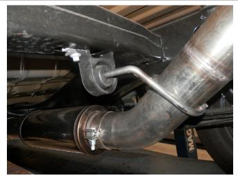
**Step 6.** Loosely install the Over Axle Pipe Assembly using the supplied clamp. Engage the welded hanger to the rubber insulator.
