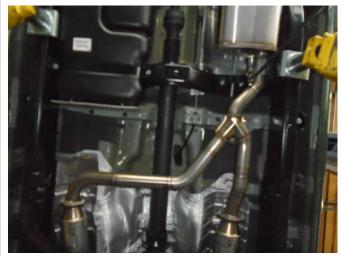
**Step 3.** Begin installing your new system by loosely attaching the Inlet Pipe Assembly to the drivers side catalytic converter outlet using the OEM hardware. Loosely slip the inlet of the Y-Pipe Assembly over the Inlet Pipe outlet and loosely secure with the supplied clamp. Loosely secure the Y-Pipe flange to the passengers side catalytic converter using the OEM hardware.
