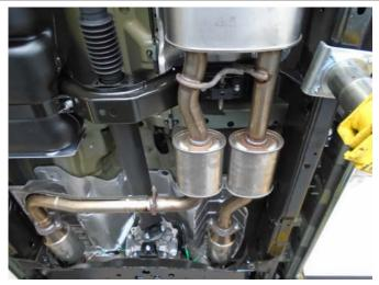
**Step 1.** Remove the OEM system by first unbolting both inlet assemblies from the front catalytic converters.
