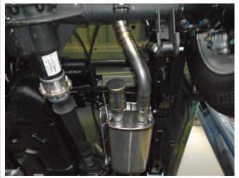
**Step 4.** Install the Muffler Assembly by engaging the welded hangers to the rubber isolators. The system comes with the option of using the NDT chamber or the Block Off Cap for a more aggressive exast note. Loosely attach the Muffler Assembly inlet to the Y-Pipe outlet using the supplied clamp.
