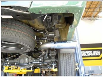
**Step 5.** Loosely install the Over Axle Pipe and Tail Pipe Assembly using the supplied clamps.
