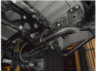
Install the Tail Pipe to the Over Axle Pipe outlet using the supplied clamp. Engage the hanger to the OE rubber insulator.
