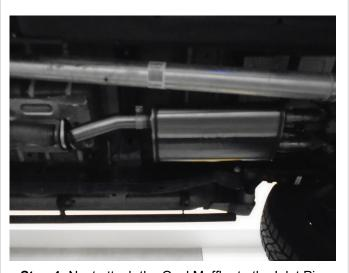
**Step 4:** Next attach the Oval Muffler to the Inlet Pipe with the supplied 2.50" clamp. This exhaust system is configured to allow the user to tune the sound. For a more moderate exhaust sound install the U-pipe Assy and the 4.00" NDT Chamber (as shown) using the suppled 2.50" clamps. For a more aggressive sound see configuration chart below.
