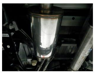
**Step 3.** Attach the Muffler Assembly to the Inlet Pipe Assembly with a supplied 3.00" clamp, fit the hanger into the rubber insualtor.
