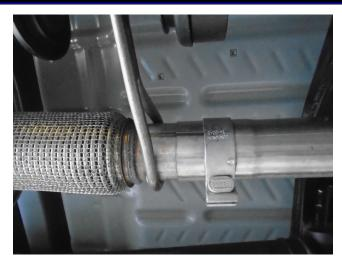
**Step 1.** To remove the OEM exhaust system, loosen the clamp attaching the systems inlet pipe to the catalytic converter outlet pipe. Disengage all welded hangers from the OEM rubber insulators. Do not discard the OEM fasteners or damage the rubber insulators as they will be needed to mount your new MAGNAFLOW system.
