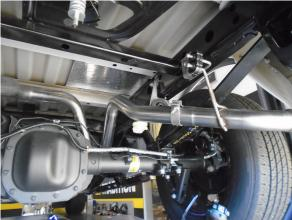
**Step 5.** To allow for the installation of a dual outlet system on a single outlet vehicle you will have top mount the supplied Hanger Brackets to existing holes in the factory frame rails using the supplied fasteners (8mm bolt and panel nut) as shown in the photos. Once completed you can now slide the Tailpipe assemblies onto the Over Axle pipes and fasten with the supplied 2.50" clamps and mount the hangers to the installed hanger brackets using the supplied rubbber insulators.
