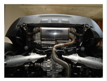
**Step 3** Next, attach the Muffler Assembly to the Inlet Pipe using the supplied 2.25" clamp. Engage the welded hangers to the rubber insulators. It may be necessary to loosen the pipe junction between the catalytic converter and the OE resonator to allow for proper tip alignment.
