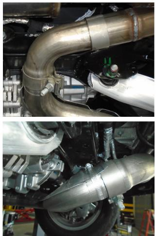
**Step 2**: Begin installing the new exhaust system by attaching the specific Inlet Pipe (2.0L or 1.5L engine) to the cut OE outlet using the supplied 2.18/2.36 clamp. Use the supplied hose clamp to re-attach the heatshield if necessary.
