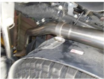
**Step 7:** Loosly install the two Tailpipe Extension Pipes using the supplied clamps. The longer, three bend pipe will be for the drivers side.
