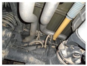
**Step 2:** To remove the system you will need to either cut the OE system with a Sawzall or similar cutting tool, or remove the rear shock absorber attached to the rear differential. The system may now be removed.
