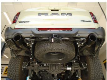
**Step 8:** Loosely attach each Tail Pipe Assembly to the Tailpipe Extension Pipes using the supplied clamps. Locate the welded hangers to the rubber isolators.
