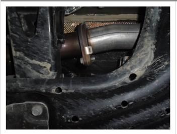
**Step 1:** Begin removal of your OE system by first removing the nuts at both inlet flange junctions.
