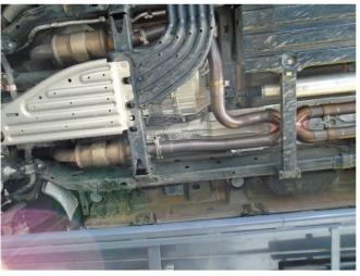
**Step 3:** Begin installing your new system by first loosely attaching the Inlet Pipe Assembly to the catalytic converter outlet flange using the supplied hardware. Next, attach the X-Pipe Assembly by slipping the Inlet Pipe Assembly outlet to the X-Pipe Assembly inlet. Loosely secure using teh supplied clamp. loosely attach the X-Pipe Assembly inlet flange to the catalytic converter outlet using the supplied hardware.
