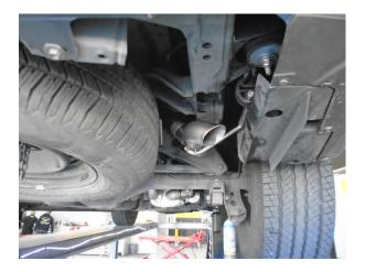
Complete the assembly by loosely attaching the Tailpipe Assembly to the Mid-Pipe using a supplied 2.50" clamp and inserting the hanger into the rubber insulator. Once a final position has been chosen for the new exhaust system, evenly tighten all clamps from front to rear using the torque specifications on page one of the instructions. Inspect all fasteners after 25-50 miles of operation and re-tighten if necessary.
