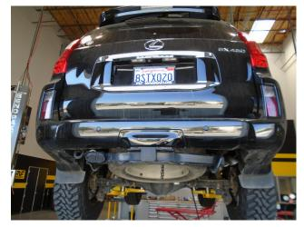
Once a final position has been chosen for the new exhaust system, evenly tighten all clamps from front to rear using the torque specifications on page one of the instructions. Inspect all fasteners after 25-50 miles of operation and re-tighten if necessary.
