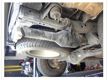
Working front to rear disengage all welded hangers from the rubber insulators and remove the system. (Retain the insulators as they will be needed to mount the new MAGNAFLOW system.) hardware.
