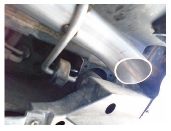
Using the OE rubber insulators install the tailpipe assemblies to the Over Axle Pipe fitting the hangers into the installed hanger brackets.
