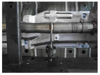
**Step 3.** Attach the Extension Pipe Assembly to the Inlet Pipe Assembly with a supplied 3.00" clamp. Engage the welded hanger to the rubber insulator.
