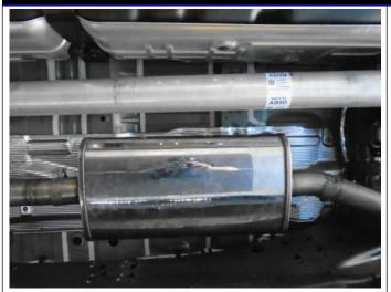
**Step 4.** Loosely attach the Muffler Assembly to the Extension Pipe Assembly with a supplied 3.00" clamp. Engage the welded hager to the rubber insulator.
