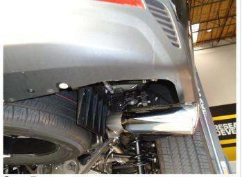
**Step 7.** Complete the installation by attaching the Tailpipe Assembly to the Pipe Assembly using the Supplied 3.00" clamp. Engage the welded hanger to the rubber insulator.
