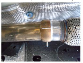
**Step 2.** Unfasten the clamp attaching the OE inlet pipe assembly to the catalytic converter. Do not damage or discard the inlet pipe clamp or rubber insulators as they will be re-used to mount the new system.
