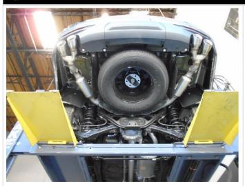
**Step 1.** To remove the OE exhaust system you will need to remove the spare tire, heat shield and sway bar.
