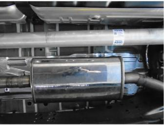
**Step 5.** Attach the Muffler Assembly to the Inlet Resonator Assembly with a supplied 3.00" clamp. Engage the welded hanger to the rubber insulator.
