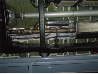
**Step 4.** To begin, fasten the Inlet Resonator Assembly to the outlet of the OE system using the OE clamp and by fitting the welded hanger to the rubber insulator (Leave all clamps and fasteners loose for final adjustment of the complete system.)
