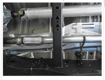
**Step 3.** Working front to rear disengage the hangers from their rubber insulators and remove the complete exhaust from the vehicle.
