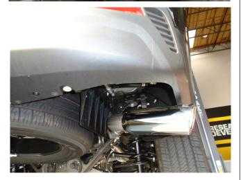
**Step 5.** Complete the installation by attaching the Tailpipe Assembly to the Pipe Assembly using the Supplied 3.00" clamp. Engage the welded hanger to the rubber insulator.
