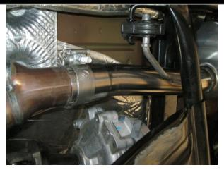
**Step 1.** To remove the OEM exhaust system, unbolt the clamps at the catalytic converter and over-axle pipe. Disengage the welded hangers from the rubber isolators and remove the components. You may need to temporarily remove the transmission skidplate to aid in removal and installation.
