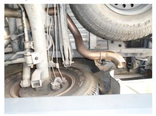
Using the supplied rubber insulator and 2.50" clamp install the Tailpipe Assembly to the Muffler by fitting the hanger into the installed hanger bracket.
