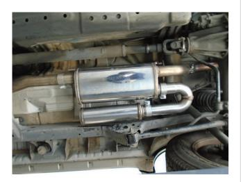
**Step 4:** Next attach the Oval Muffler to the Inlet Pipe with the supplied 2.50" clamp. This exhaust system is configured to allow the user to tune the sound. For a more moderate exhaust sound install the U-pipe Assy and the 4.00" NDT Chamber (as shown) using the suppled 2.50" clamps. For a more aggressive sound use the Block off Pipe in place of the U-Pipe & NDT Chamber using the supplied 2.50" clamp. The MF block Off Pipe are not used in this configuration (Not shown).
