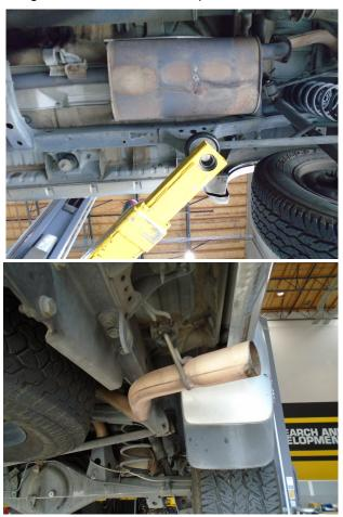
**Step 2:** Working front to rear, disengage all welded hangers from the rubber insulators and remove the system. (Retain the rubber insulators as they will be needed to mount the new MagnaFlow system.)
