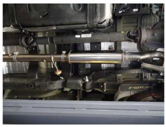
Step 5: At this point, if required, add the 19.25" Extension Pipe using a supplied clamp. Next, Loosely attach the Extension Pipe Assembly(has welded hangers attached)followed by the Muffler Assembly using the supplied clamps. Engage the welded hangers to the rubber insulators.
