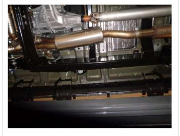
Step 2: Next loosen the clamp rearward of the OEM resonator. Detach all welded hangers from the rubber insulators. The system may now be removed. Be sure to retain all mounting hardware as it will be needed to install your new MAGNAFLOW system
