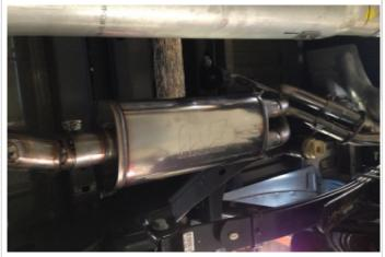
Step 3. Install the Muffler Assembly to the Inlet Pipe Assembly using the supplied 3.00" clamp.
