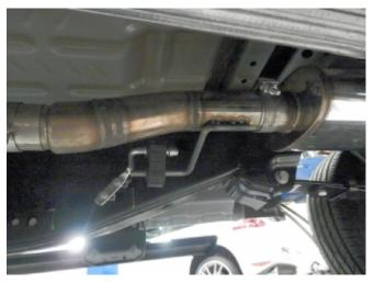
Step 2. . Install the new system by attaching the Inlet Pipe Assembly to the OEM catalytic converter outlet pipes using the existing clamp and hardware. Locate the welded hanger to the rubber insulator. Leave all clamps and fasteners loose for final adjustment of the complete system once installed.
