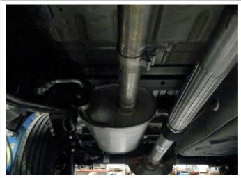
Step 1. To remove the OEM exhaust system, loosen the clamp attaching the systems inlet pipes to the catalytic converter outlet pipes. Disengage all welded hangers from the OEM rubber insulators. Do not discard the OEM fasteners or damage the rubber insulators as they will be needed to mount your new MAGNAFLOW system.
