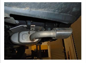
**Step 1:** To remove the OE exhaust assembly unfasten the hardware at the flange. While supporting the exhaust extract the hangers from the rubber insulators (retain rubber insulators as they will be reused).
