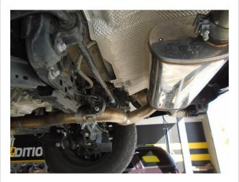
**Step 3:** Next, attach the Muffler Assembly to the Resonator using the supplied 2.50 Clamp and by fitting the hanger into the rubber insulator.
