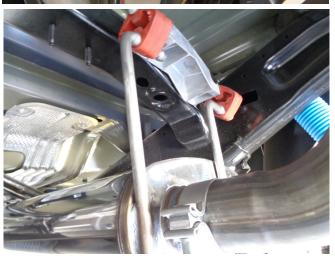
Step 4: Locate the welded hangers to the rubber insulators. Leave all clamps loose for final adjustment of the complete syste once installed.
