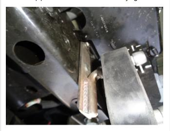
Step 6: On the driver side attach the bracket assembly with the bolts and washers provided.
