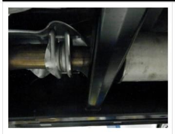
Step 1. To remove the OEM exhaust system, you will first need to unbolt the muffler assembly from the flange junction as shown.
