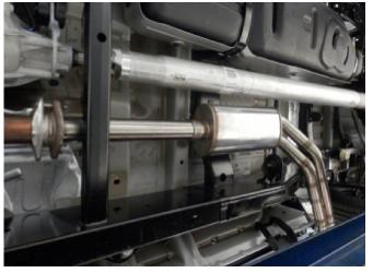
Step 6. Install the Muffler Assembly and loosely secure using the supplied 3.00" clamp. Attach the Hanger Bracket Assembly to the welded hanger using the supplied rubber insulator.
