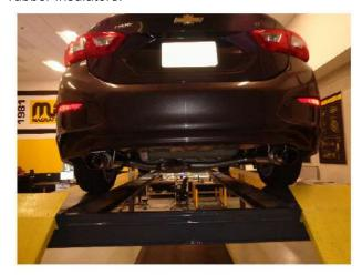
**Step 6:** Once a final position has been chosen for the new exhaust system, evenly tiligen all clamps from front to rear using the torque specifications on page one of these instructions. Inspect all fasteners after 25-50 miles for operation and re-tighten if necessary.
