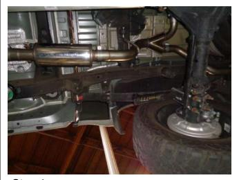
Step 4. Next loosely attach the Y-Pipe Assembly to the Muffler Assembly using the supplied clamp. Engage the welded hangers to the rubber insulators.
