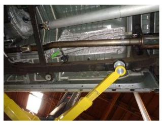
Step 3. Only the Crew Cab Long Bed configuration will require the supplied 12.5 Extension Pipe, Install this to Inlet Pipe Assembly if required using the supplied 3.00" clamp then attach the Muffler Assembly to the Extension Pipe. If the 12.5" Extension Pipe isn't used attach the Muffler Assembly directly to the Inlet Assembly with a supplied 3.00" clamp.
