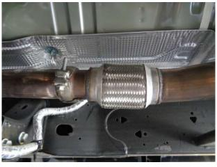
Step 2. To begin, fasten the Inlet pipe assembly to the outlet of the OE system using the OE clamp assembly and by fitting the welded hanger into the rubber insulator (Leave all clamps and fasteners loose for final adjustment of the complete system.)
