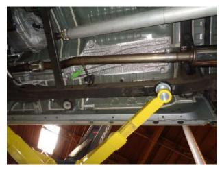
Step 3. Only the Crew Cab Long Bed configuration will require the supplied 12.5 Extension Pipe, Install this to the Inlet Pipe Assembly if required using the supplied 3.00" clamp then attach the Muffler Assembly to the Extension Pipe. If the 12.5" Extension Pipe isn't used attach the Muffler Assembly directly to the Inlet Assembly with a supplied 3.00" clamp.
