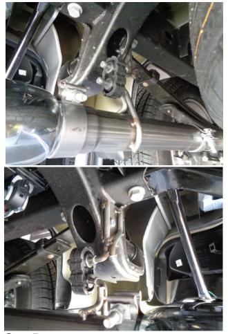
Step 5. As this vehicle was not setup for dual exhaust from the factory, hanger brackets will need to be installed. Install the hanger brackets on the rear frame section using the supplied fastener hardware as shown
