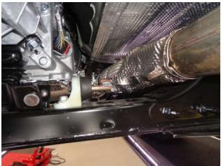
Step 1. To remove the OEM exhaust system, you can then disengage the welded hangers from the rubber insulators and remove the tailpipe assy. Unfasten the clamp attaching the OEM inlet pipe assembly to the catalytic converter. Do not damage or discard the inlet pipe clamp or rubber insulators as they will be re-used to mount the new system. Disengage the inlet pipe assembly hanger and remove the exhaust from the vehicle.
