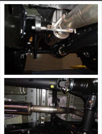
Step 3. Next loosely attach the Tailpipe Assembly to the Muffler Assembly using the supplied clamp. Engage the welded hanger to the rubber insulator.
