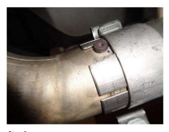
**Step 2:** To install the MagnaFlow Y-Pipe Assembly slide the inlet onto the OE outlet making sure to align the slot with the peg on the outlet pipe. Secure with the supplied 3.00" clamp.
