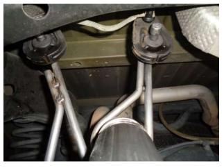
**Step 3:** insert the welded hangers into the rubber insulators
