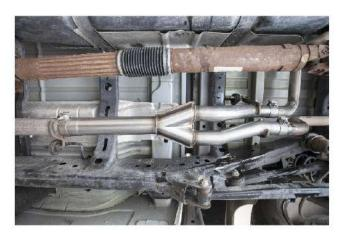
**Step 4:** Finish by fitting the OE tailpipes into the Y-Pipe Assembly by indexing the alignment pegs and securing with the supplied 2.25" clamps. Once a final position has been chosen for the new exhaust component, evenly tighten all clamps from front to rear using the torque specifications on page one of these instructions. Inspect all fasteners after 25-50 miles for operation and re-tighten if necessary.
