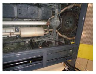
**Step 1.** Begin removal of the OE muffler by loosening the three clamps attaching the muffler to OE system. Disengage the hangers from the rubber insulators and remove the muffler. Do not discard or damage the rubber insulators as they will be used to install the new system.
