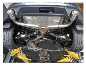
**Step 4.** Next attach the Y-Pipe Assembly to the Muffler Assembly using the supplied 3.00" clamp. Install the two Tail Pipe Assemblies in a similar fashion using the supplied 2.50" clamps. Locate the welded hangers to the rubber insulators.
