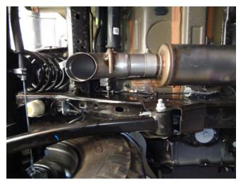
Step 4: Finish by Installing the turn down tip using the supplied clamp and fitting the hanger into the rubber insulator.
