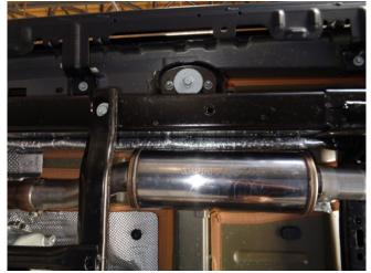
Step 3: Begin installation of your new MAGNAFLOW system by attaching the Resonator Assembly to the catalytic converter outlet using the OEM clamp. Keep all fasteners and clamps loose until final adjustment.
