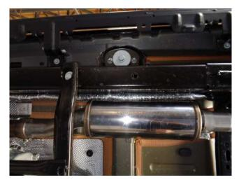
Step 3: Begin installation of your new MAGNAFLOW system by attaching the Resonator Assembly to the catalytic converter outlet using the OEM clamp. Engage the welded hanger to the rubbe insulators. Keep all fasteners and clamps loose until final adjustment.
