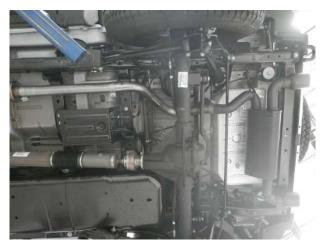
Step 5: Next loosely install the Over-Axle and Muffler Assemblies using the supplied clamps. Locate all welded hangers to the rubber insulators.
