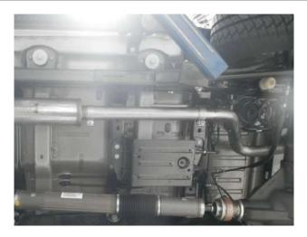
Step 4: The included Extension Pipe is required for the four door model only. It is to be installed between the Resonator Assembly and the Over-Axle Pipe. if you have the two door model this pipe may be discarded.
