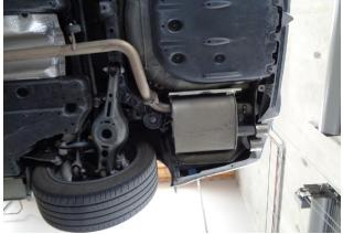
Step 1. To remove the OE exhaust system begin by unfastening the 2 bolt flanges, one located at the front of the vehicle (behind the catalytic converter assy) and one at the rear (by the muffler). Working front to rear disengage the hangers from the rubber insulators and remove the exhaust. Do not damage the rubber insulators and retain front flange hardware as they will be used to install the new exhaust system.
