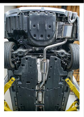
Step 2. Begin installation of the MagnaFlow system by attaching the Resonator Assembly to the outlet of the catalytic converter using the OE fasteners. Next, attach the Muffler Assembly using the supplied 2.50" clamp and engaging the hangers into the rubber insulators. (Leave all clamp and fasteners loose for final adjustment of the complete system.)
