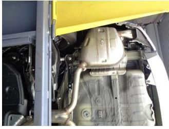
**Step 1.** To ease removal of the OE exhaust system unbolt the cross braces located on the underside the vehicle and remove. Begin by unfastening the rear muffler assembly at the flange located at the rear of the vehicle in front of the driver side muffler. Extract the hanger from the rubber insulators and remove the assembly. Do not discard or damage the OE fasteners or rubber insulators as they will be used to install the new system.
