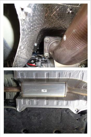
Step 2: Next unfasten the front 3 bolt flange located behind the catalytic converter, extract the hangers from the rubber insulators and remove the remaining part of the OE system.
