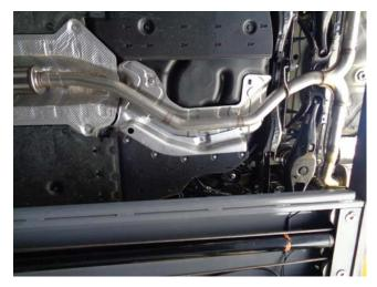
Step 4: Next use the supplied 2.250" clamp to attach the Y-Pipe Assembly to the Resonator Assembly and insert the hanger to rubber insulator.
