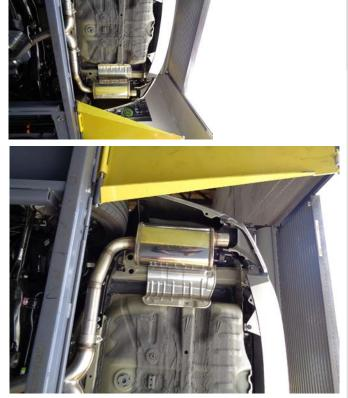
Step 5: Next use the supplied 2.50" clamps to attach the Muffler Assemblies to the Y-Pipe Assembly and insert the hangers into rubber insulators.
